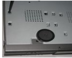
Fig 2-2 Screw in the HDD
