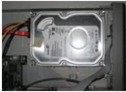
Fig 2-1 Connect the HDD
